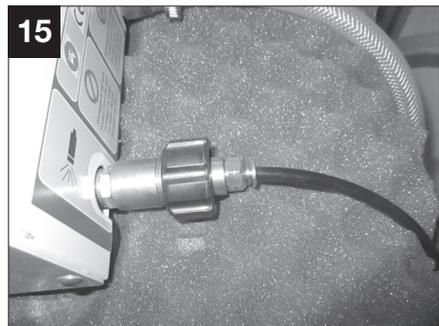
6. Make sure that the water in the centralised water system has a pressure between 2 and 5 bar (30 - 70 psi), then at this point open the valve to power the machine.
